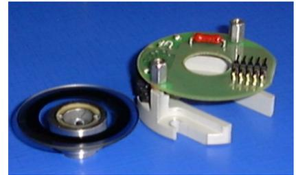
The encoder **A42M** is similar to the ERO 1222 type encoder (Heidenhain) in electrical parameters, mounting and overall dimensions.
